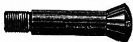
Round Face Wire Chuck Fitted to any Lathe.
