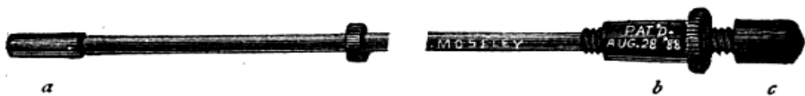
Fig. 44. Stepping Device. a —rests in chuck and should be slightly less than diameter of work. b —tightens in rear of draw-in spindle. c —turning this regulates depth of step.
