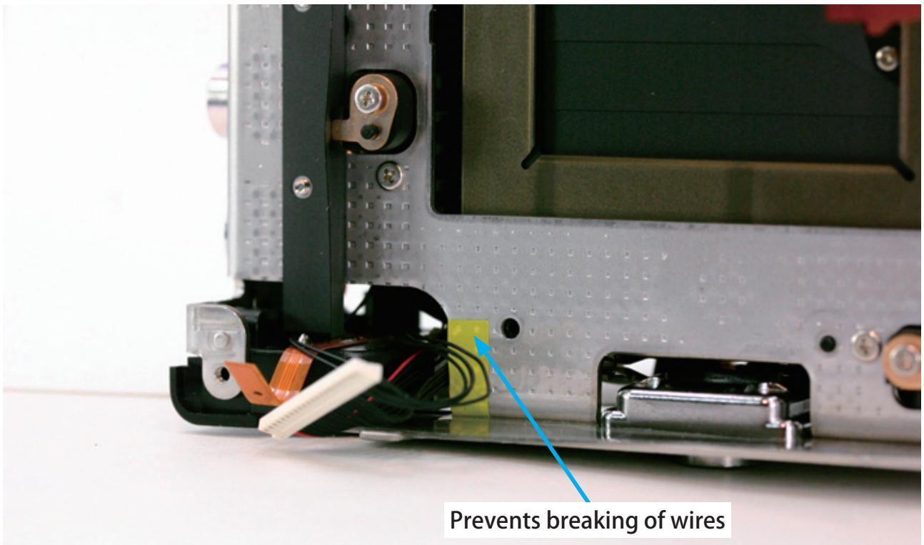
Prevents breaking of wires
