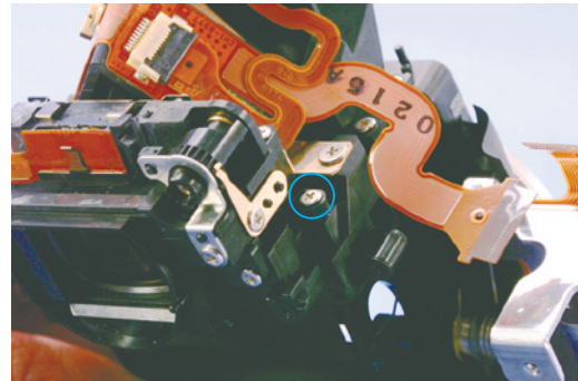
Fig. 087 Eyepiece Ass'y Removal 2
