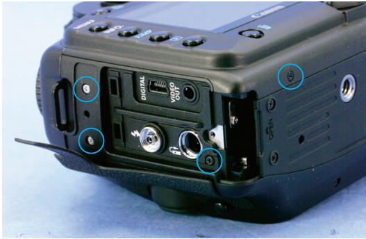
Fig. 023 Interface Cover Removal 1
