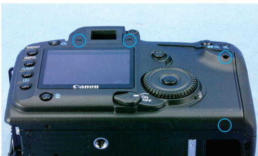
Fig. 025 Back Cover Removal 1
