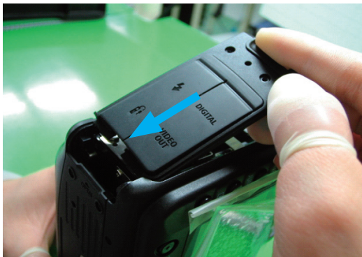
Fig. 030 Interface Cover Installation
