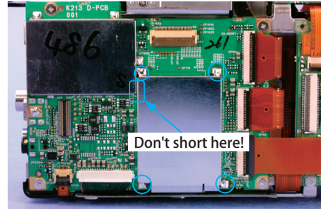
Fig. 045 Digital PCB Shield Cover Removal
