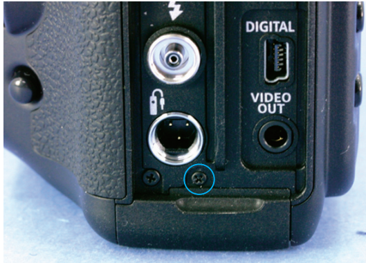
Fig. 017 Date Battery Case Removal 1
