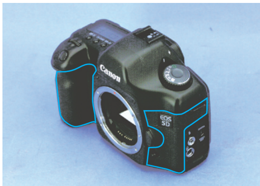
Fig. 019 Rubber Covers Removal 1
