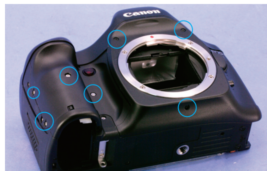
Fig. 027 Front Cover Removal
