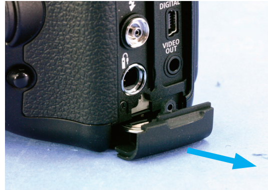
Fig. 018 Date Battery Case Removal 2
