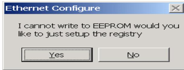
Click on **YES** to store the IP address in the registry so that software from the Pewin Pro Suite can recognize the Ethernet accessory as an available PMAC Device. Afterwards, a dialog box displays requesting a card. This number is changed from 0 to another number only when using multiple PMACs simultaneously from a single host. When doing so, the additional PMACs must be programmed with a unique IP address.
