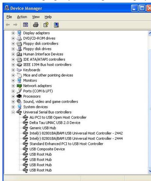
If Delta Tau UMAC USB 2.0 Device is not on the list, the device driver has not been installed. If there is a red x through that line or a yellow exclamation point through that line, then Windows had a problem installing the device.
