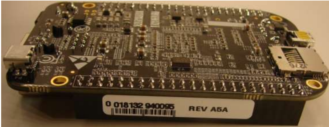
Figure 73. Third Phase Serial Number and Revision Location
