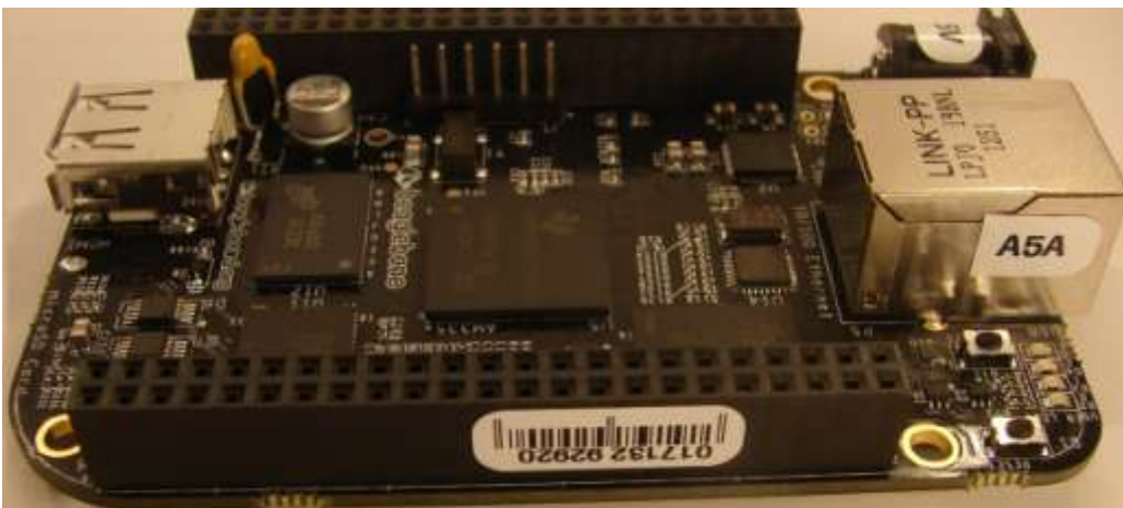
Figure 72. Second Phase Serial Number and Revision Location
