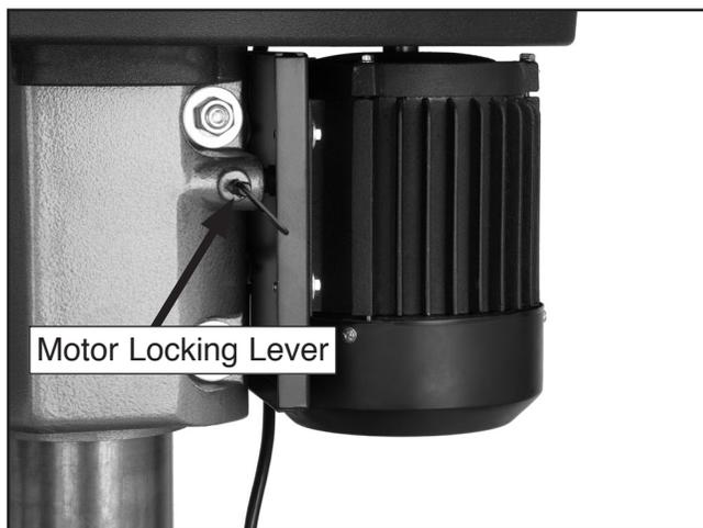
**Figure 28.** Motor locking lever.
