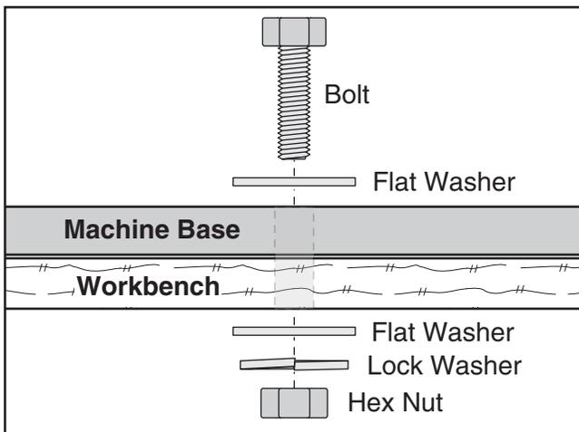
Figure 8. Example of a through mount setup.
