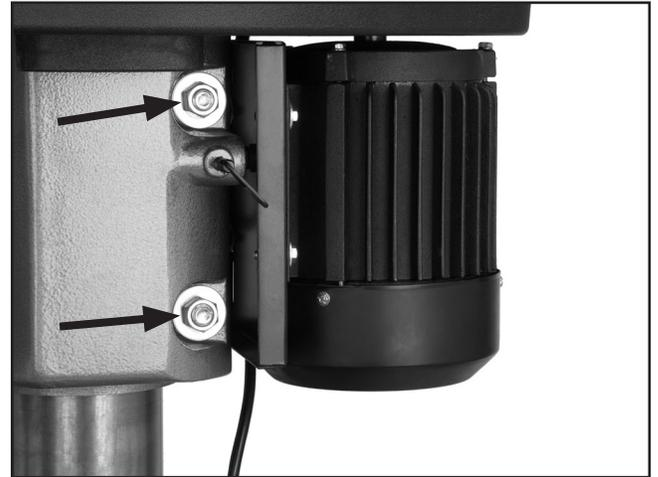
**Figure 27.** Head locking nuts.
