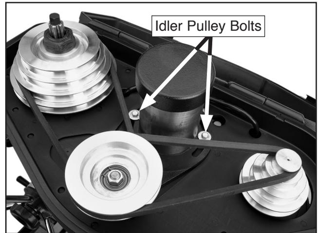
**Figure 29.** Pulley system.
