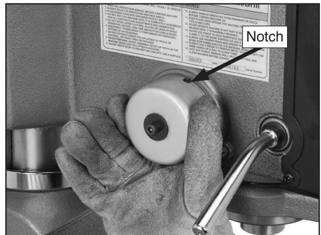
Figure 40. Adjusting spring tension.
