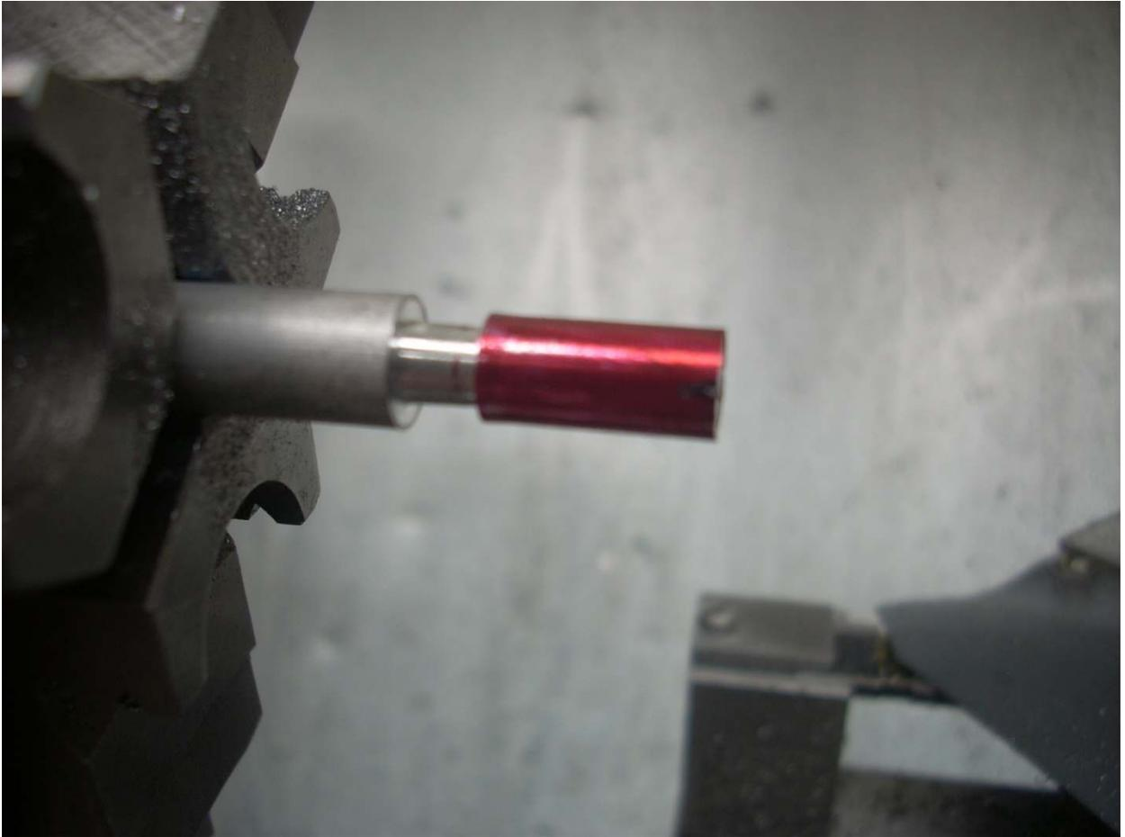
Now the all critical step – coat the surface to be threaded with Dykem.
