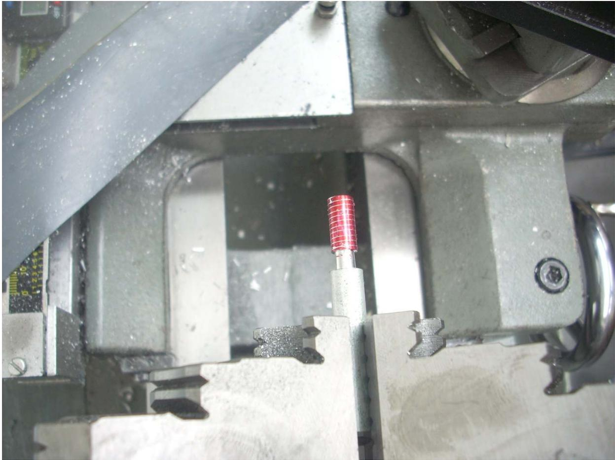
I move the cutter so it just touches the part and zero both my cross slide and compound dials. Then I back out the compound and move the apron over so the cutter is to the right of the part. And finally, I turn the compound's dial back to zero.
