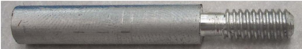
Single point turning of a thread can seem extremely difficult until you successfully do it. One area of frustration is knowing how deep to go with the cutter. The procedure that Frank shared with me removes much of this frustration.
