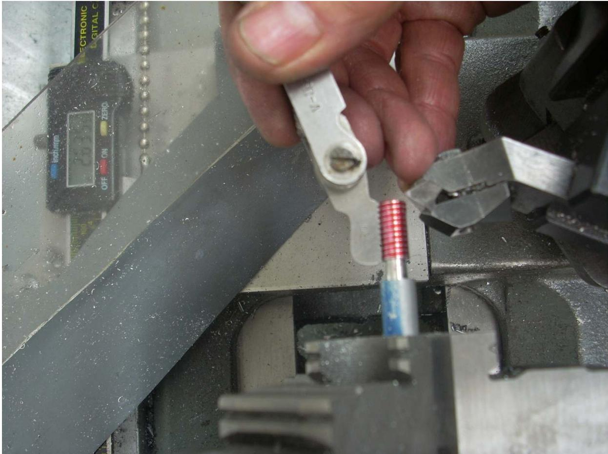
Using my thread gage, I verify that I am cutting 20 threads per inch.
