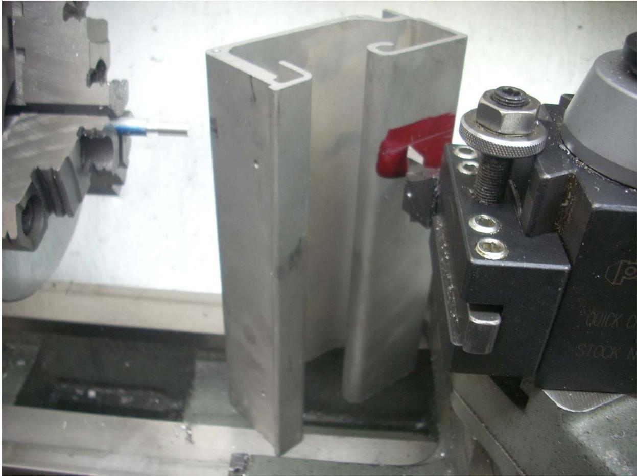
I own a Diamond<sup>®</sup> tool holder which comes with a threading cutter. I use my fancy height gage to set the cutter's height to the lathe's center of rotation.
