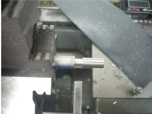
My stock is about 0.3" in diameter so I first turn it down to the nominal diameter of 0.250". The spec says it can be between 0.246" up to 0.254" for a class 2A thread.
