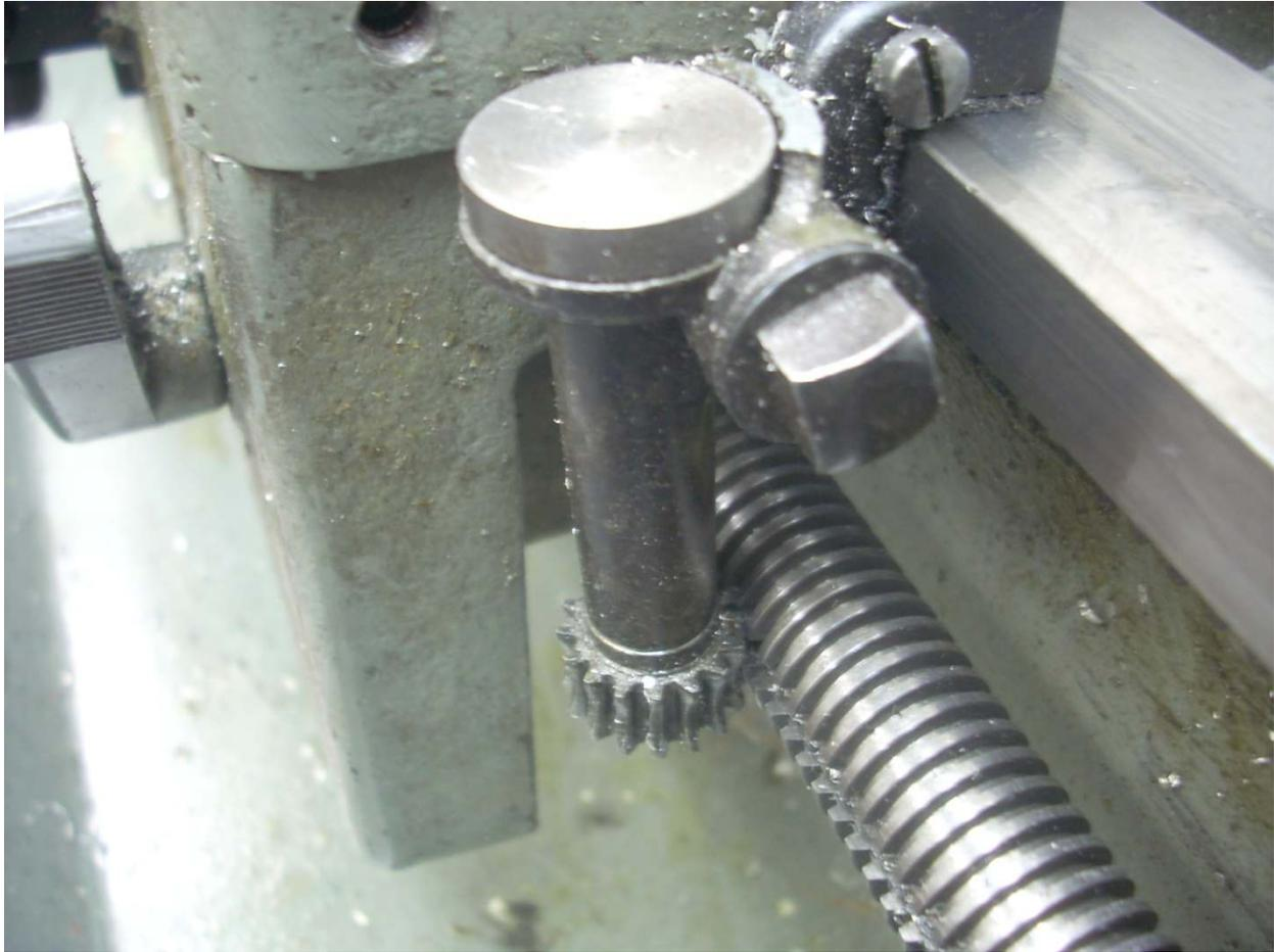
I am now ready to set up the lathe for threading. The “clock” is engaged. It will tell us when to lock in the split nut.
