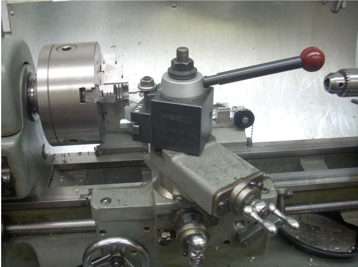
Next I set my compound to 29.5 degrees. This provides 0.5 degrees of clearance for my cutter which has the necessary 60 degree included angle point.
