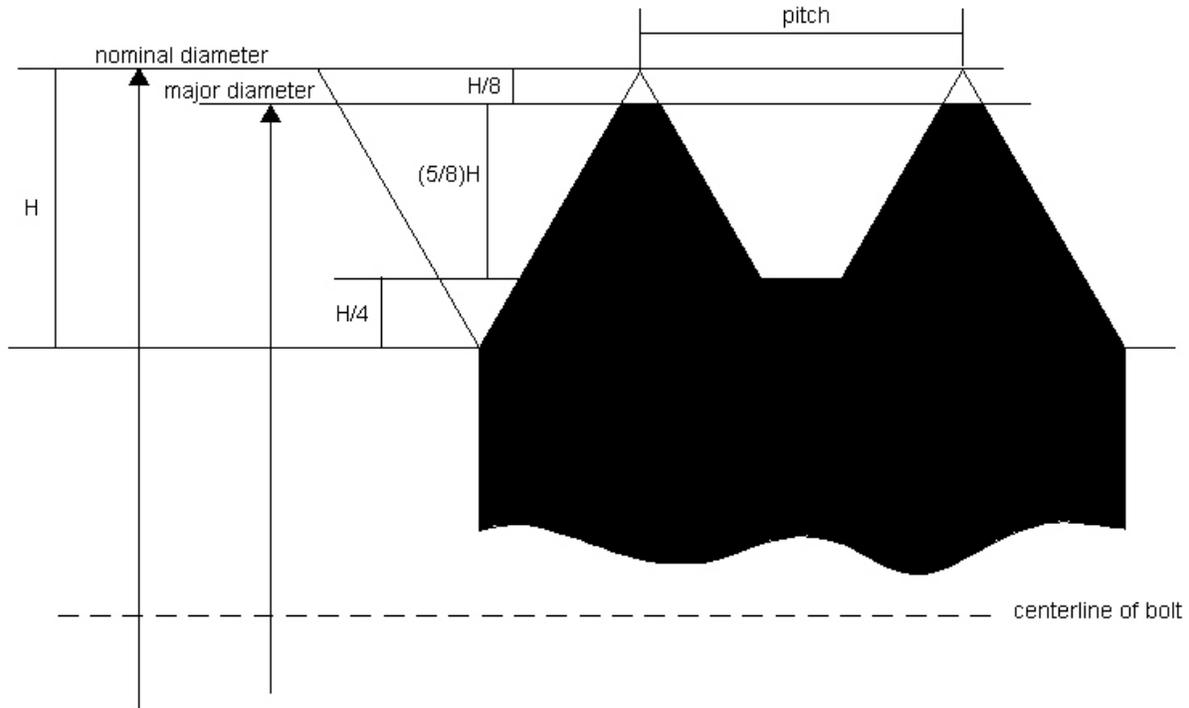
The center of the bolt is shown as that dashed line at the bottom. Not drawn to scale, we have the profile of the thread. The outer most surface of the thread is defined as the major diameter.
