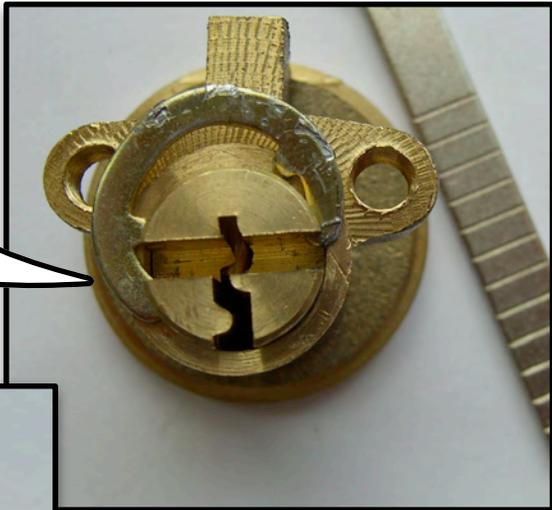
THE CIRCLIP HOLDS THE PLUG IN PLACE. HOWEVER, EVEN WITH THE CIRCLIP REMOVED THE PLUG WILL NOT COME OUT BECAUSE THE PINS ARE STILL BLOCKING THE REMOVAL OF THE PLUG
