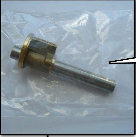
TIP: USE A PLASTIC BAG WHEN REMOVING THE PLUG FOLLOWER. THIS WILL CONTAIN THE SPRINGS AND PINS WHEN THEY GO SPROING! (AND THEY WILL!)
