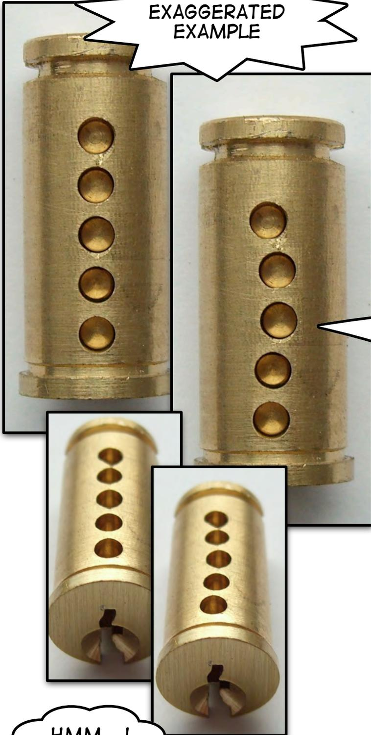
LOCK PICKING WORKS BECAUSE OF A VULNERABILITY CREATED BY MECHANICAL TOLERANCES IN THE MANUFACTURE OF LOCKS. SMALL MISALIGNMENTS IN THE PIN CHAMBERS, CHAMBERS THAT ARE MISSHAPEN (OVAL), AS WELL AS MISSHAPEN PINS WILL CREATE WHAT IS CALLED THE BINDING EFFECT (EXPLAINED NEXT).
