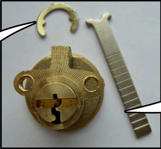
IN ORDER TO REMOVE THE PLUG, THE PIN STACKS MUST ALL BE LIFTED TO THE SHEAR LINE. THIS CAN BE DONE WITH THE CORRECT KEY, BY PICKING THE LOCK, OR WITH A THIN METAL SHIM
