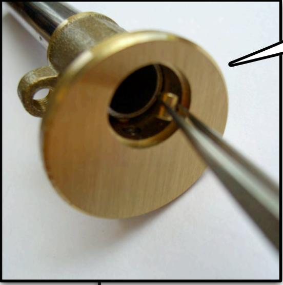
ONCE ALL PIN STACKS ARE INSTALLED, YOU CAN USE THE PLUG TO REPLACE THE PLUG FOLLOWER. IT IS JUST LIKE REMOVING THE PLUG, BUT IN REVERSE!
