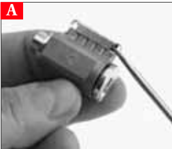
A Using a screwdriver or other small edge carefully pry off the steel cap from the top of the cylinder
