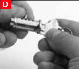
D Load new bottom pins into the plug that correspond to the new key combination
