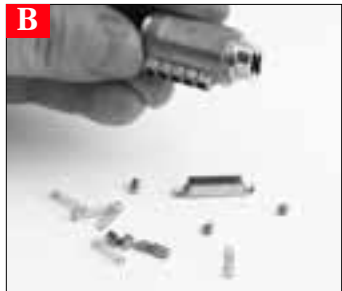
B Dump contents from the top of the cylinder (springs, top pins and bottom pins)
