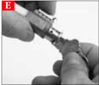
E Re-insert the plug back into the housing and push the plug follower back out. Finally, re-insert the C-Clip cylinder retaining ring onto the back of the plug
