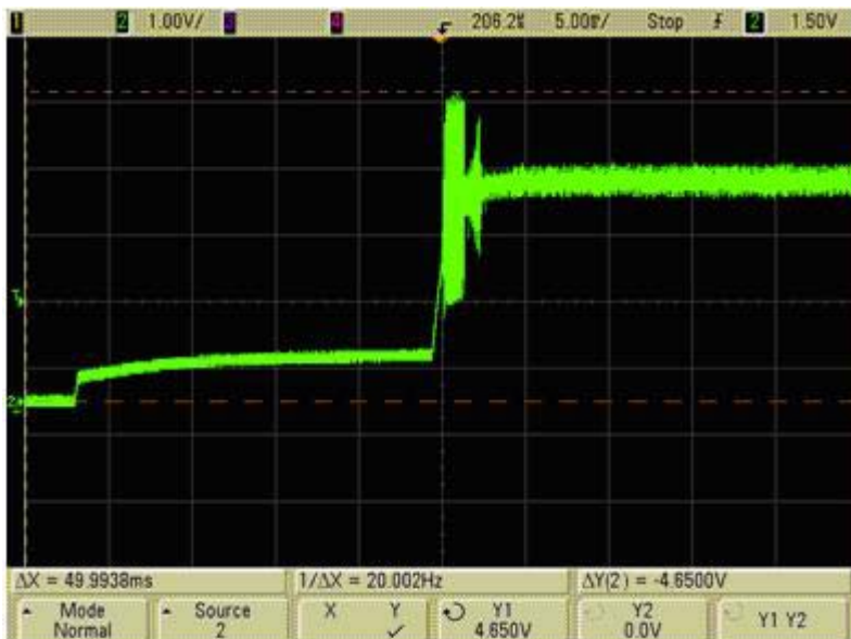
Figure 10. Input Voltage Overshoot >4V (Bad)
