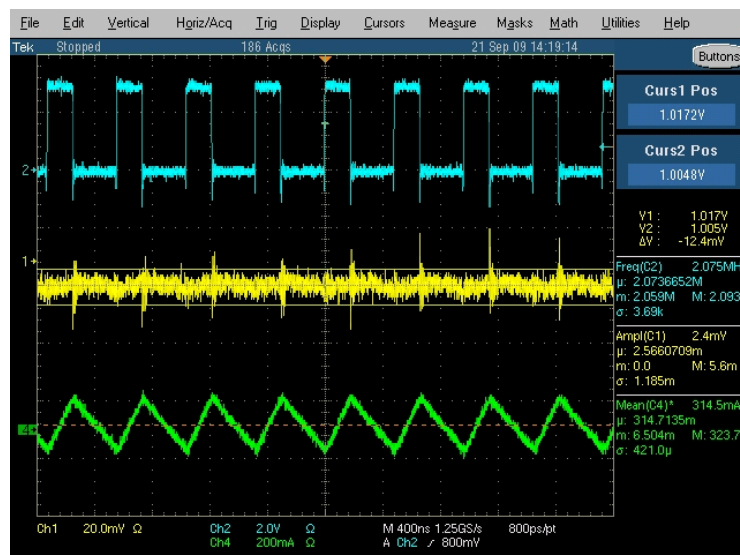
Figure 12. L=GLK2510P-2R2M, C=Ceramic 4.7 \mu F 0805 X5R TDK (Ripple 12.4mV)
