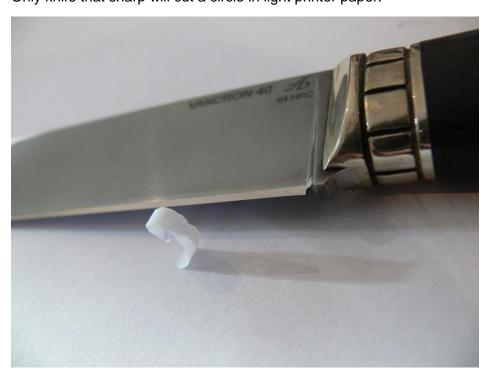
**Cigarette paper test** done on Tally-Ho or Rizla Green rolling paper (approx. 17gsm). The test has two gradations: longitudinal and cross push-cut.
