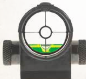
#113: Spirit Level front globe sight. (As seen from the muzzle)
