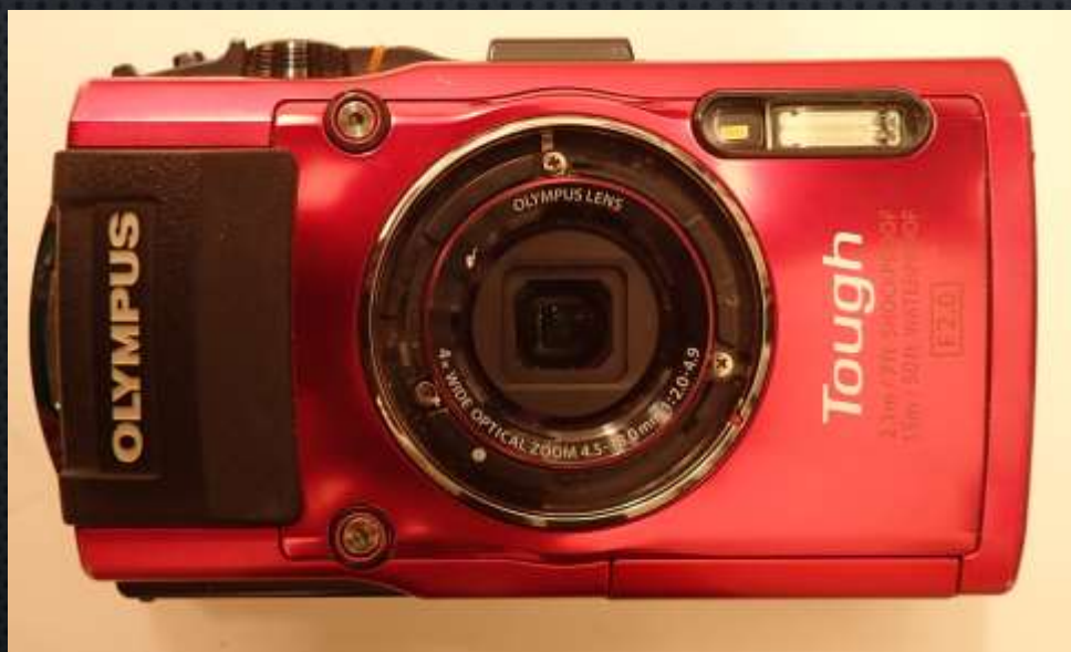
Camera with bayonet ring removed
