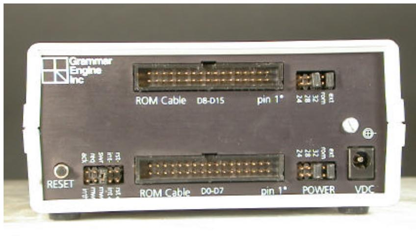
Note the dual set of ROM cable headers and power headers. Each set configures one of the two 8 bit units inside the dual PromICE.
