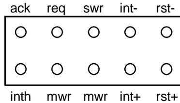
The Optional Connect Header is on the PromICE back panel. It has auxiliary signals that allow you to control the target system from the host, as well as additional features that allow PromICE to interact with the target. These signals are as follows:
