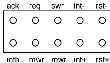
**int- and int+:** (outputs) These interrupt signals are driven by PromICE whenever the HDA bit is set in the AI status register. This occurs during AI communications, or when caused by a host command. Both polarities of the signal are provided. They are driven by a 74LS125 tri-state buffer. The signals are driven when asserted and are tri-stated when not asserted. This allows these signals to be shared by other sources.
