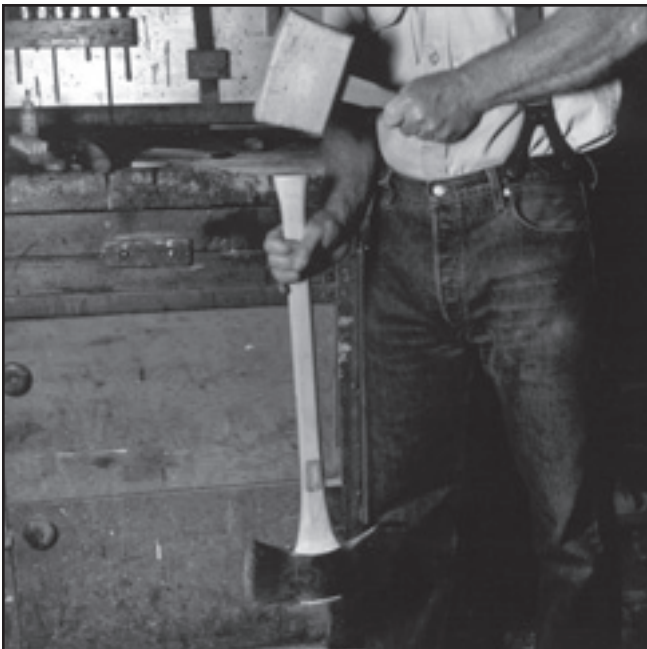
Figure 52—Time for the final fit. Drive the head on by striking the bottom of the handle. You can often tell when the head will move no farther by the solid sound of the strike.
